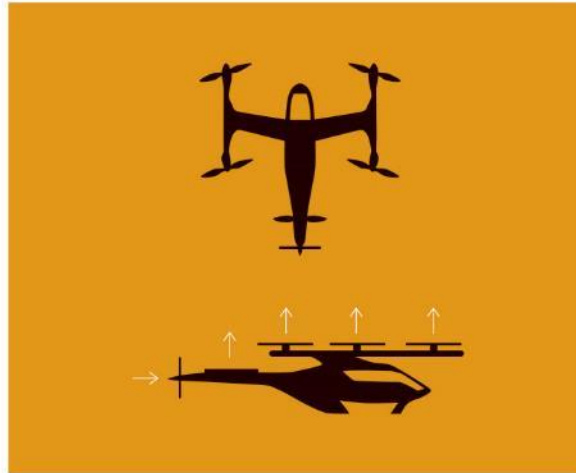
LIFT AND CRUISE: One group of vertical rotors lift the aircraft and another set provides forward thrust; wings boost cruise energy efficiency.
