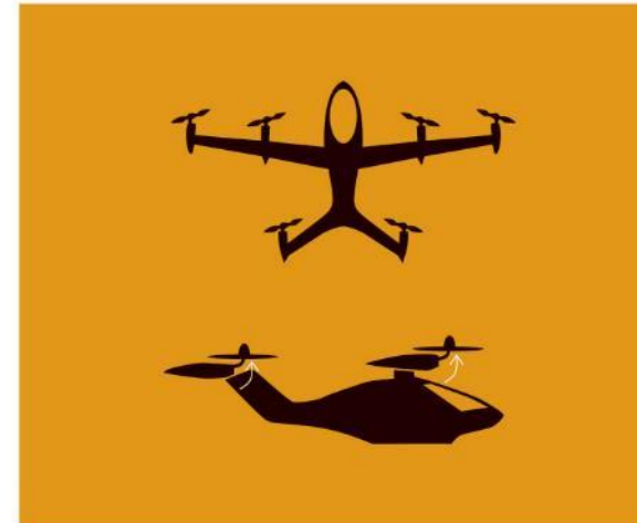
VECTORED THRUST: Tilting propulsors transition the aircraft from liftoff thrust to forward thrust; wings boost cruise efficiency.
