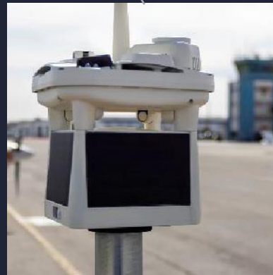
Intellisense MWS Surface Weather, Ceiling, Visibility
