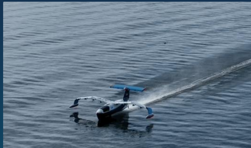
REGENT's ¼ scale seaglider prototype effortlessly glides through waves on its hydrofoil before taking off
