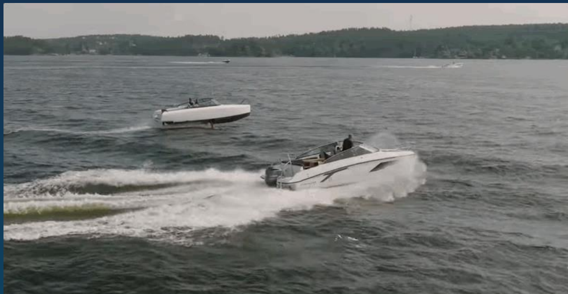
Wave tolerance comparison of hydrofoil vs conventional hull boat
